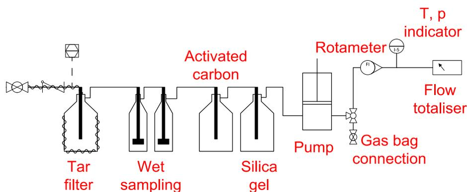
Fig. 4. Sampling train used in pilot-plant tests.
