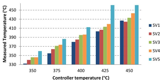
Fig. 6. Temperature measured at the top of the sorbent bed as a function of the space velocity and the temperature set point (SV1 =  $150 \text{ h}^{-1}$ , SV5 =  $750 \text{ h}^{-1}$ ).
