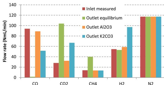
Fig. 7. Gas flow rates experimental results measured at SV of  $150 \text{ h}^{-1}$  and  $400^\circ\text{C}$ , and equilibrium composition.
