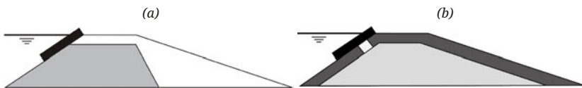
Figure 11.2. Scenarios for deployment of BresDefender: (a) stop overflow and arrest breach growth, and (b) reduce stability reduction by blocking infiltration of water at damaged levee sections (Janssen, Schmets, Hofland, Dado, & Jonkman, 2020).
