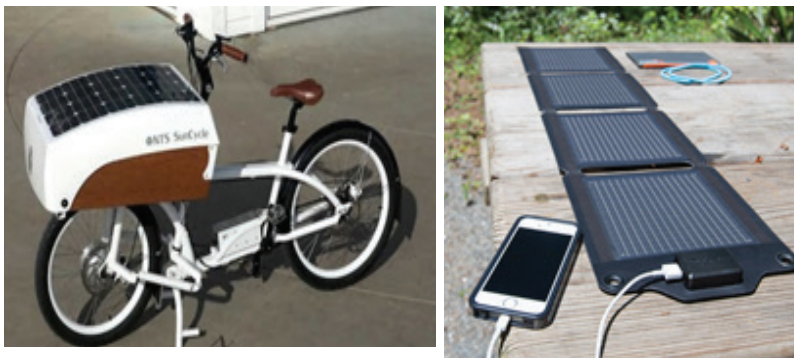
FIGURE 1.7: LEFT: NTS SUN CYCLE IS POWERED WITH A 60W BUILT-IN SOLAR PANEL (APPROXIMATELY 4 SQUARE FEET) AND CHARGING SYSTEM, 2014 (TREEHUGGER, 2014). RIGHT: PV-POWERED CHARGER FOR OUTDOOR USE, 2011-2013 (ATLANTA TRAILS, 2015).
