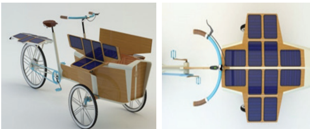
FIGURE A.9: SUN BIKE IS AN ELECTRIC TRICYCLE, WHICH IS POWERED USING THE SOLAR PANELS THAT ARE LOCATED ON THE COVER OF THE CARGO. SOURCE: TUVIE, 2015.
