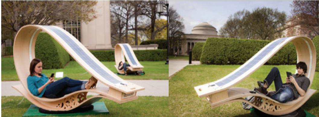
FIGURE A.15: SOFT ROCKERS (2011) ARE PV-POWERED CHARGING STATIONS, LOCATED OUTDOORS. THEY ARE DESIGNED TO RECHARGE ELECTRONICS, WHILE RELAXING OUTDOORS. THEY USE THE HUMAN POWER OF BALANCE TO CREATE A SOLAR TRACKING SYSTEM OF 35 WATT. DESIGNED BY SOFT ROCKERS TEAM (2011). SOURCE: ARTS.MIT.EDU, 2015.
