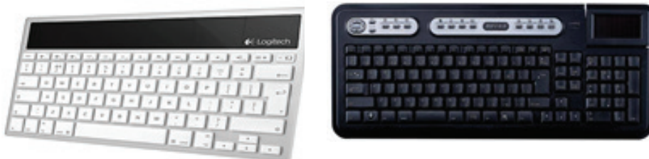
FIGURE A.26: LEFT IMAGE: LOGITECH PV-POWERED KEYBOARD (2010), MODEL K760 WIRELESS BLUETOOTH KEYBOARD FOR THE MAC. SOURCE: NOTEBOOK CHECK, LOGITECH, 2012, MACWORLD, 2014. RIGHT IMAGE: BSKBW015B PV-POWERED WIRELESS KEYBOARD BY BUFFALO JAPAN (2008). IT OPERATES IN FREQUENCY 2.4 GHZ WITH 10 METERS RANGE. SOURCE: NEWLAUNCHES, 2014.
