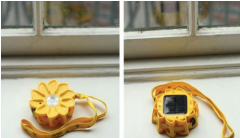
FIGURE 6.17: LITTLE SUN LIGHT PLACED ON THE WINDOWSILL. LEFT PICTURE: THE FRONT SIDE OF THE PRODUCT. RIGHT PICTURE: THE BACKSIDE OF THE PRODUCT INCLUDING THE PV CELL.
