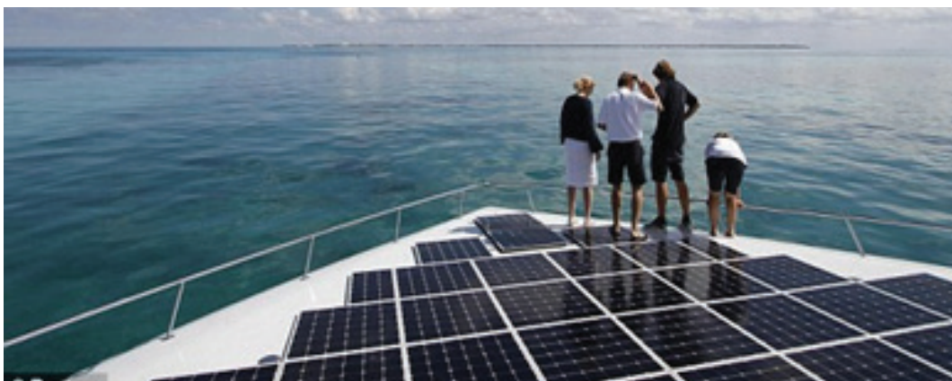
FIGURE A.11: THE TYRANOR PLANET SOLAR CATAMARAN (2010-2012), 102FT LONG, 29FT WIDE AND 25FT HIGH, IS THE LARGEST PV-POWERED SEA VESSEL. SOURCE: DAILYMAIL, 2015.
