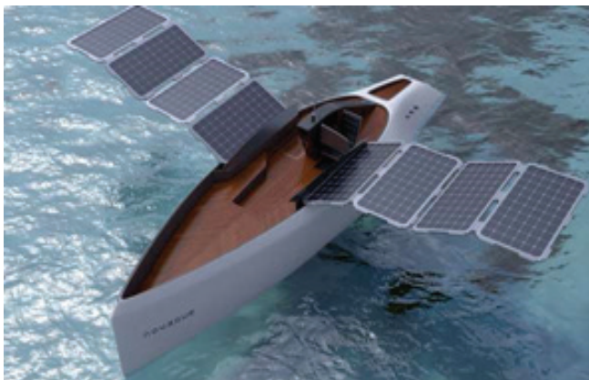
FIGURE A.14: PV YACHT BY NOVAGUE STUDIO IS A CONCEPT PRODUCT (2009). THE SOLAR PANELS FITTED ON THE BOAT OPEN ON BOTH SIDES LIKE WINGS. SOURCE: SOLAR FEEDS, 2015.
