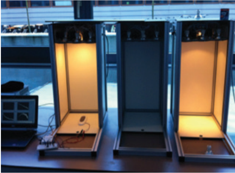
FIGURE 4.7B: THE EXPERIMENTAL SET-UP THAT WAS USED FOR THE MEASUREMENTS OF THE LAMPS' SPECTRUM (APOSTOLOU ET AL., 2016).
