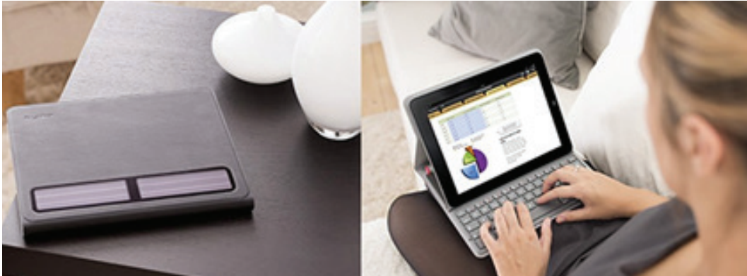
FIGURE A.24: LOGITECH SOLAR KEYBOARD FOLIO (2012) IS A WIRELESS SOLAR KEYBOARD, WHICH USES DYE-SENSITIZED SOLAR CELLS (DSSC) –THE G24 SOLAR CELL- DESIGNED TO BE USED WITH APPLE IPADS (THE IPAD 2 AND IPAD 3). THE KEYBOARD HARVESTS INDOOR AMBIENT LIGHT. IMAGE COURTESY OF G24 POWER LTD. SOURCE: GCELL, 2014.
