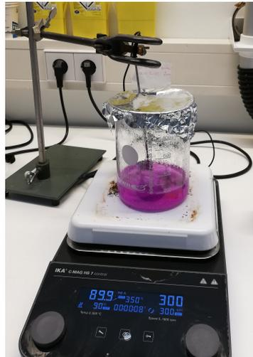
Figure 2.1: Specimen preparation set-up including a glass beaker containing PVA powder solved in distilled water and coolant covered with aluminum foil placed on a stirring plate. The place is set to heat the sample until 90°C and stirring 300 rounds per minute. A sensor is placed in the mixture to measure the temperature.
