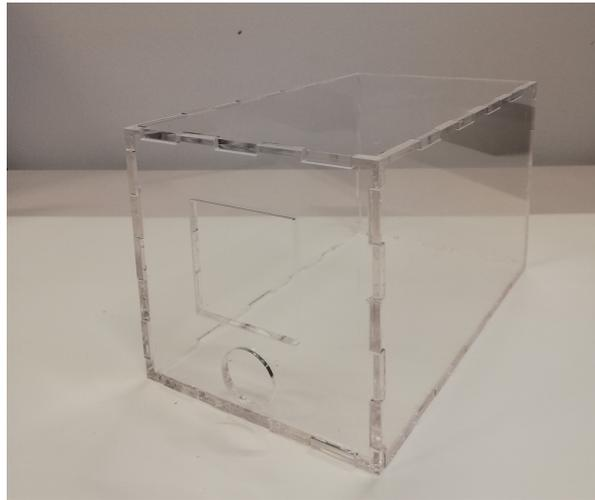
Figure 3.3: Casing of the prostate phantom model. The model is made of transparent PMMA material with 4 mm thickness. The outer dimensions of the casing conclude 120 x 120 x 208 mm. An opening is present at the front which enables needle insertion. A round opening is made for a rectal insert.
