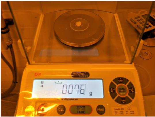
(a) Image of measuring the NaCl for the pH buffer
