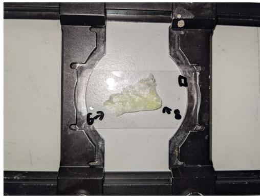
(a) Sample D in sample holder of Fluorescent microscope with pH 6 drop on the left and pH 8 drop on the right
