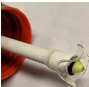
(a) Image of the final needle with sensing layer and rubber ring
