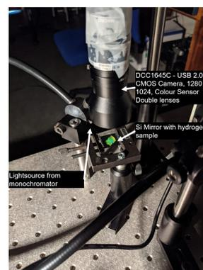
(b) Set up with Thorlabs camera, a sample and the silicon Mirror
