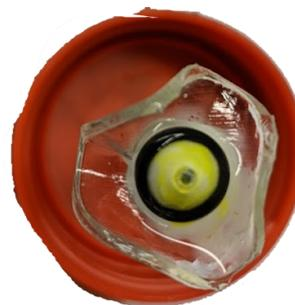
(b) Image of the final needle with sensing layer and rubber ring
