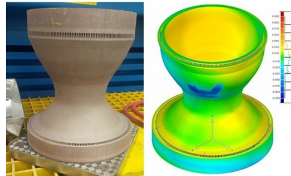
Figure 12: Example of structured light 3D scanning comparing the as-built surfaces to CAD (credits NASA).
