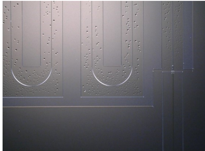
Fig. 10.1: Image from the a-Si chip fabricated using the inverted process from Fig. 8.9. Craters are clearly visible in the a-Si layer around the meandering NbTiN microstrip line.
