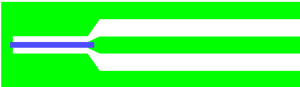
Fig. 6.3: Hybrid MKID with in blue aluminium and in green NbTiN. The thin aluminium section is shorted at one end and connects to the wide NbTiN section at the other end.
