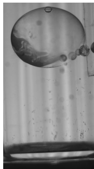
(c) Chloroform droplet in C-80 sample.
