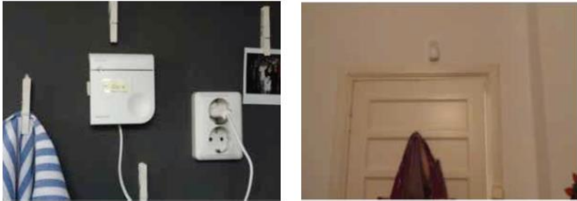
Figure 4.1: T, CO 2 , RH box (left) and movement sensor (right) as used during the Opschaler measurement campaign. (Source: Monicair report)
