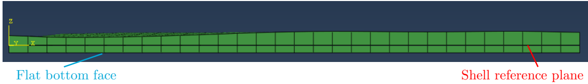
Figure 6.5: Abaqus shell offset to obtain the same ABD plane and a one-sided flat plate.
