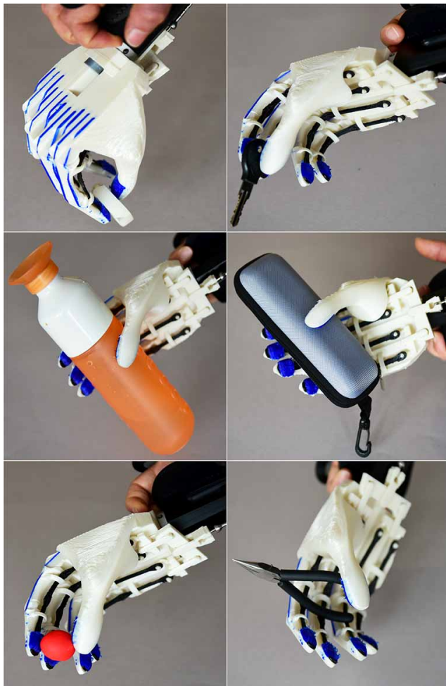
Figure 6.5: The grasping patterns. (Top left & right) Pinch grasping, (middle left & right) power grasping, (bottom left & right) and tripod grasping.
