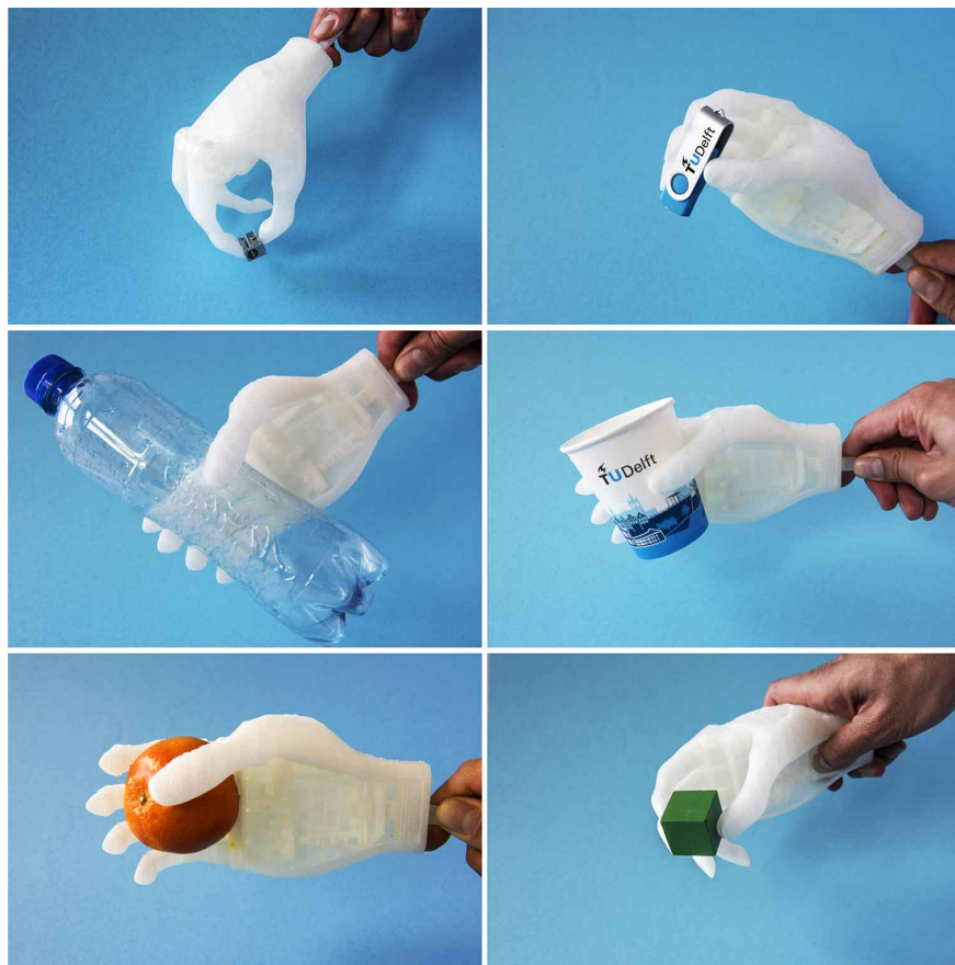
Figure 4.6: Grasping patterns. Pinch grasping ( Top left & right ), power grasping ( Middle left & right ), spherical grasping ( Bottom left ), and tripod grasping ( Bottom right ).
