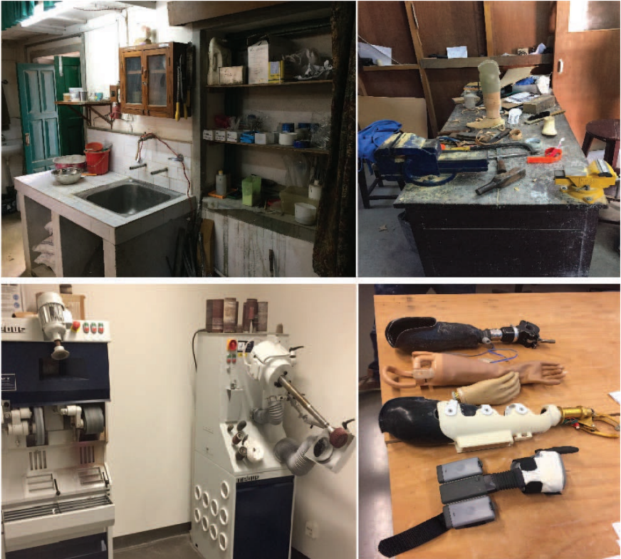
Figure 1.3: Workbench in a prosthetic workshop in Nepal (top) vs prosthetic workshop in the Netherlands (bottom). In the Netherlands state-of-the art tools and prosthetic devices are available whereas in Nepal the workbench is outdated and underequipped.
