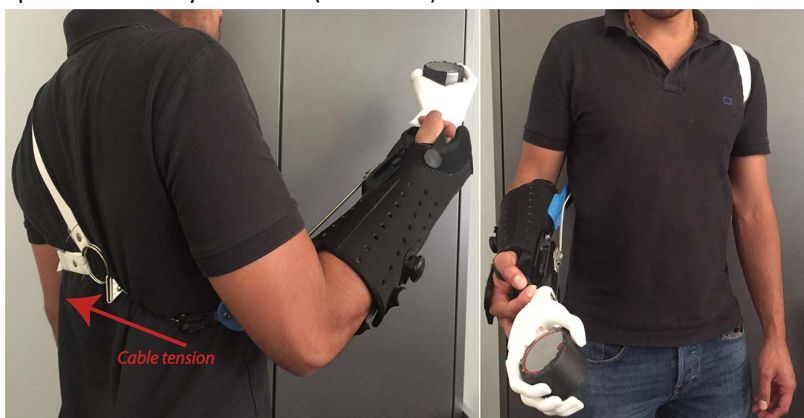
Figure 5.4: Our 3D printed prosthetic hand attached to the simulator and a figure-of-nine shoulder harness. The cable tension that is delivered by the harness and activates the prosthetic hand is depicted ( left ).
