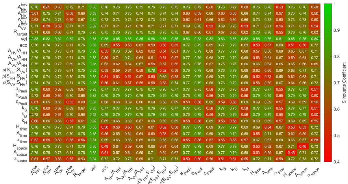
Figure 4.19: Silhouette coefficient matrix, indicating the resulted coefficient values for all possible feature pairs when clustering by k-means method with three classes
