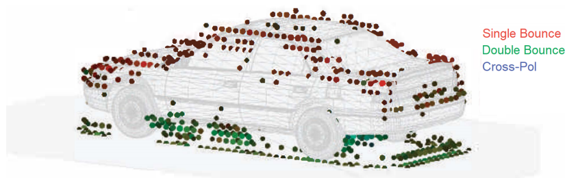
Figure 1.2: A reconstructed 3D-image of simulated X-band scattering data from Civilian Vehicle Domes (CVDOME) [43] of a Toyota Camry, applied with a Pauli basis color mapping, representing the physical interpretation of the Pauli components of all scattering points [6]
