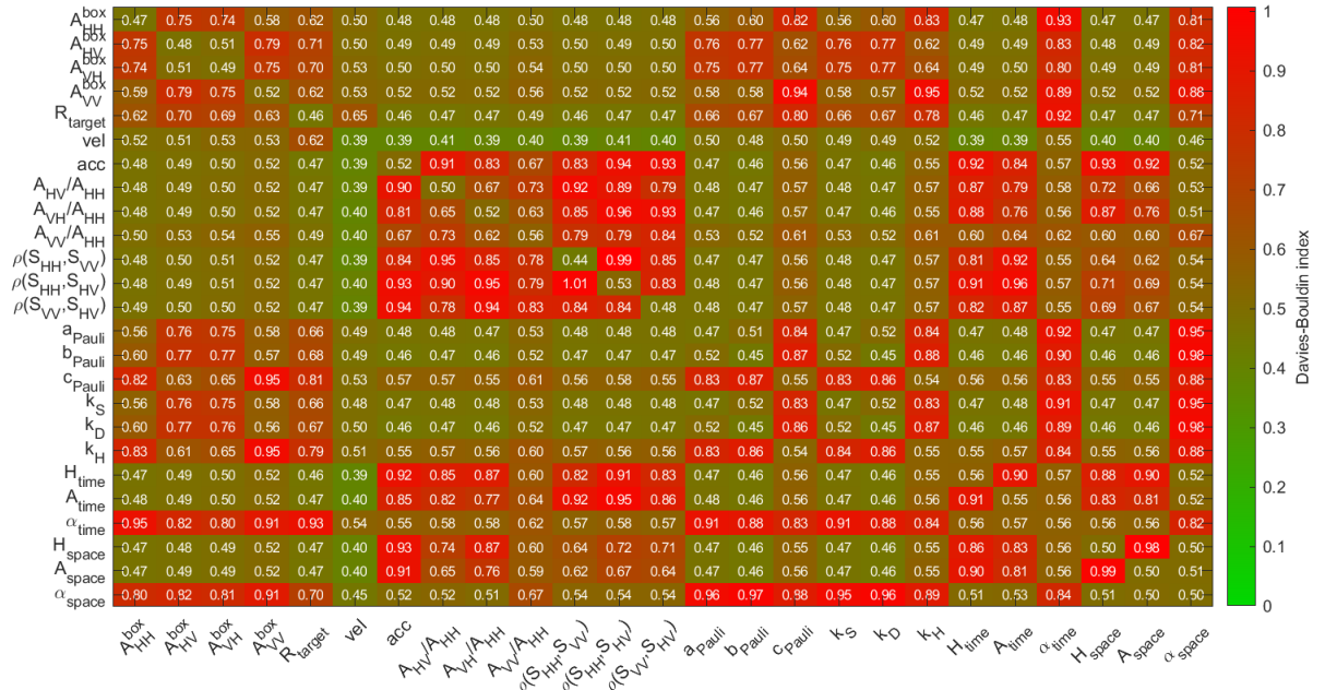
Figure 4.21: Davies-Bouldin index matrix, indicating the resulted index values for all possible feature pairs when clustering by k-means method with three classes
