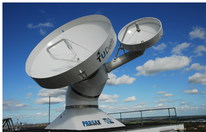
Figure 2.6: The PARSAX radar on top of the EEMCS faculty of the TU Delft
