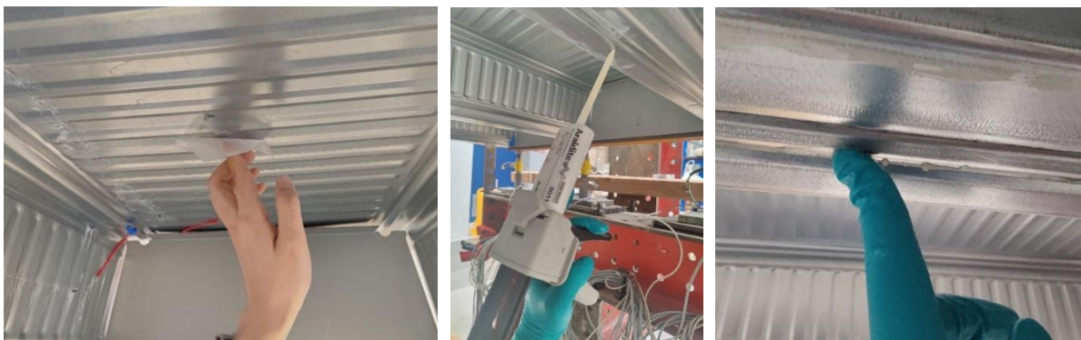
Figure 3.11. Application of two-component glue on embossments (left), application of epoxy (middle), and spreading the epoxy by hand (right).
