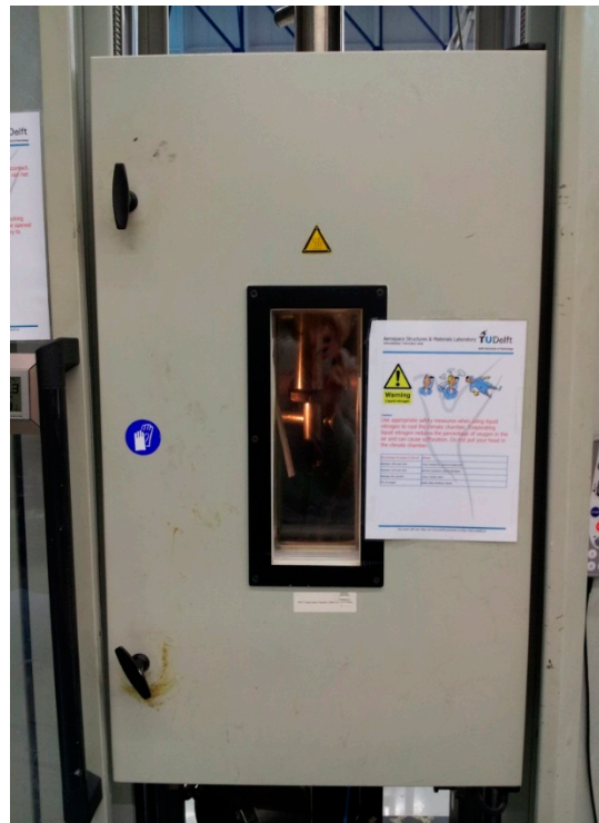
Figure 2. Climate chamber during short-beam tests.
