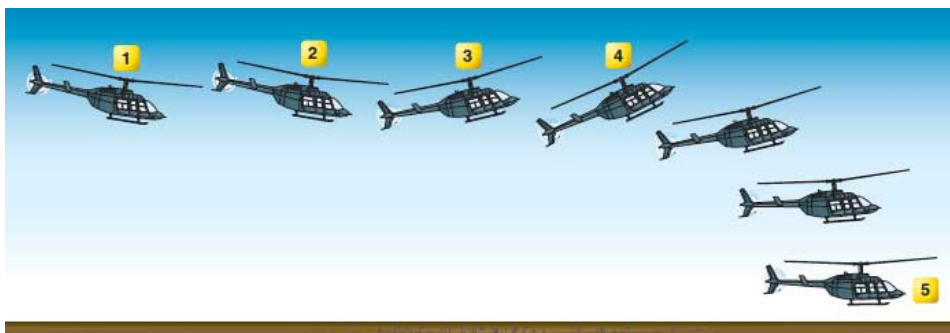
Figure 2.10 – Quick stop manoeuvre (Source: Danubewings † ).
