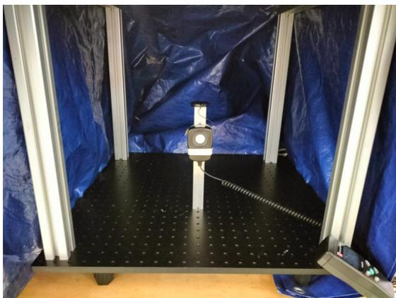
(a) Test setup for measuring light intensity
