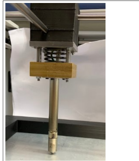
Fig. 12: A complete view of the soldering iron frame.
