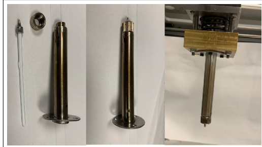
Fig. 24: The visualization of the steps to convert the machine from a sealing into a plotter machine. The sealing rod is replaced with a pen to plot a trajectory on paper instead of sealing on a material. This conversion simplifies the comparison process for error detection as the machine path can in the new setup directly be drawn on or next to the actual trajectory. An advantage of this is that it eliminates human error from the comparison process as there is no need for a human to align the machine path with the desired path. In conclusion, a pen-plotter machine will enhance error detection significantly.
