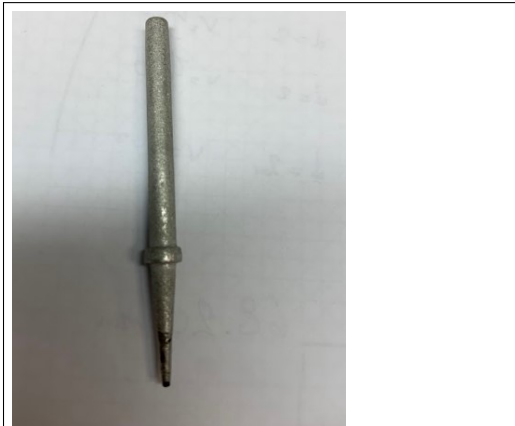
Fig. 14: Original soldering iron tip of Velleman Soldering station. The soldering iron has a sharp head and a small tip diameter.
