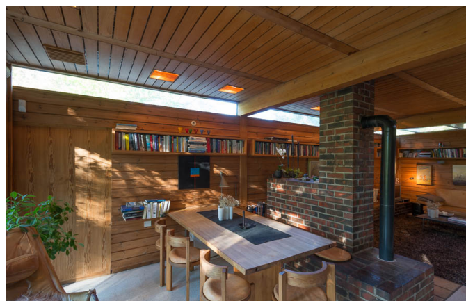
Fig. 62 - Although the facade of the villa on the street side is largely closed off, daylight is allowed to enter in the building via a horizontal opening filled with glass running from side to side. This brings in light but prevents sight from passing by neighbours (Berntsen, 2014)
