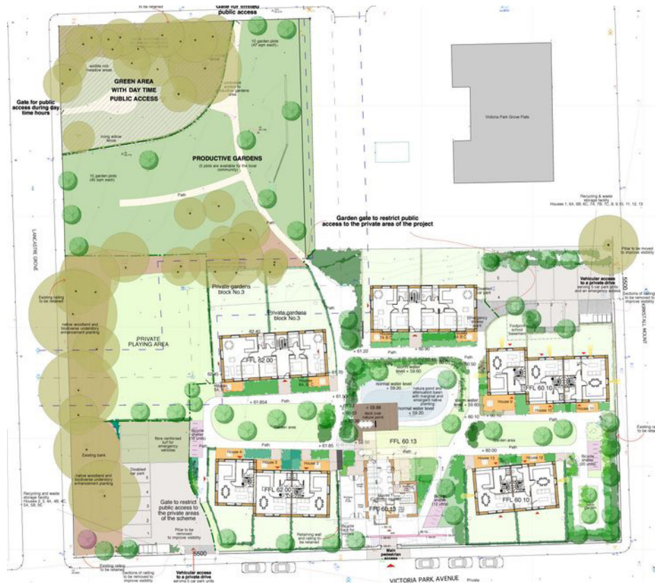
Fig. 79 – The site plan consists of five residential buildings including twenty homes, and one building that is the common house (Towards New Spitalfields, 2015)
