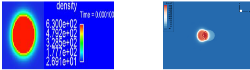
Figure 8.6: Density distribution from the work of Ping et al. [2019] and this work (left to right) for Case 1 at t = 0.1 ms
