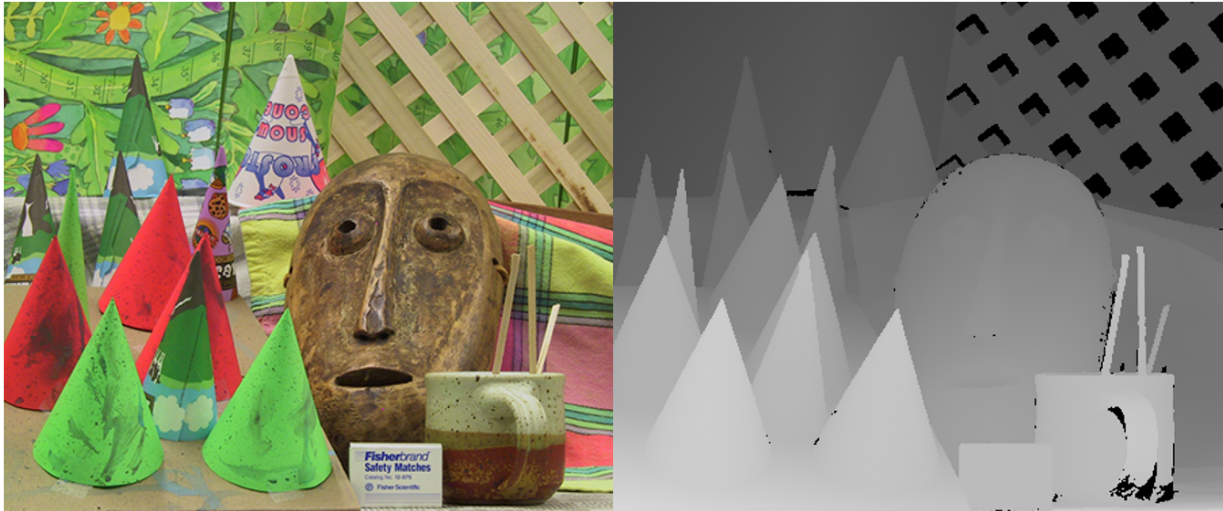
Figure 3.15: Sample scene from the Middlebury dataset with ground-truth disparity. [23]
