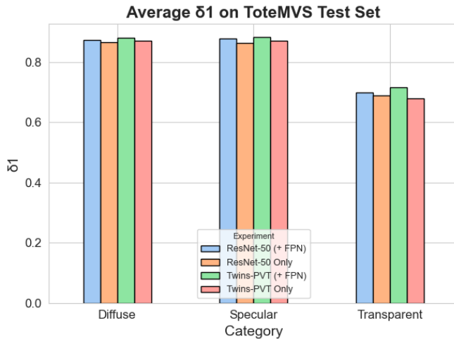
Figure 11: Effect of removing the FPN from both ViT and CNN-based backbones.
