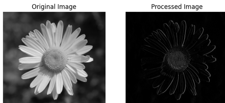
Figure 3.7: Result after applying the edge detection kernel to a sample image.
