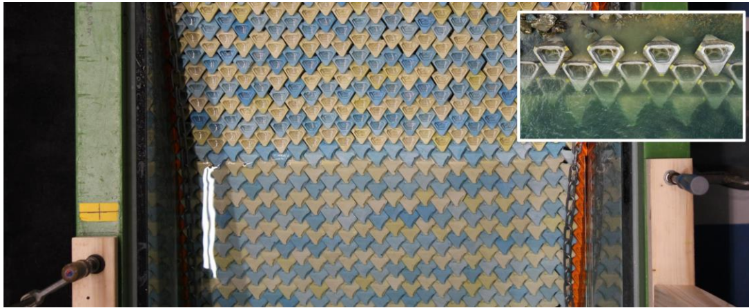
Figure 7. Standard Configuration (SD) (Molenkamp 2022) and, top right, the prototype installation in PoSD
