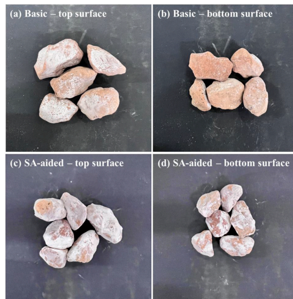
Fig. 10. The (a) top surface of RBA after basic MICP treatment, (b) bottom surface of RBA after basic MICP treatment, (c) top surface of RBA after SA-aided MICP treatment, and (d) bottom surface of RBA after SA-aided MICP treatment.
