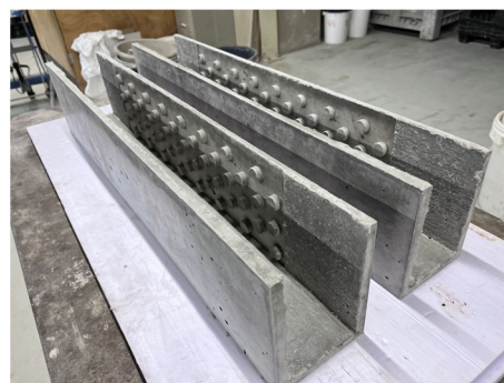
Fig. 5. Precast U-shape self-healing SHCC covers. The keys inside the cover were designed to enhance the interface bond strength between the cover and the core.
