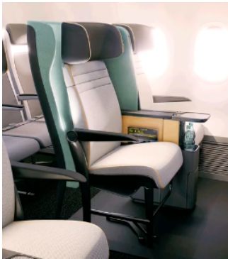
Figure 7.5: PRM seat extended for use of a passenger without a wheelchair. [12]
