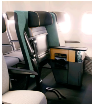
Figure 7.6: PRM seat folded for use of a passenger with a wheelchair. [12]
