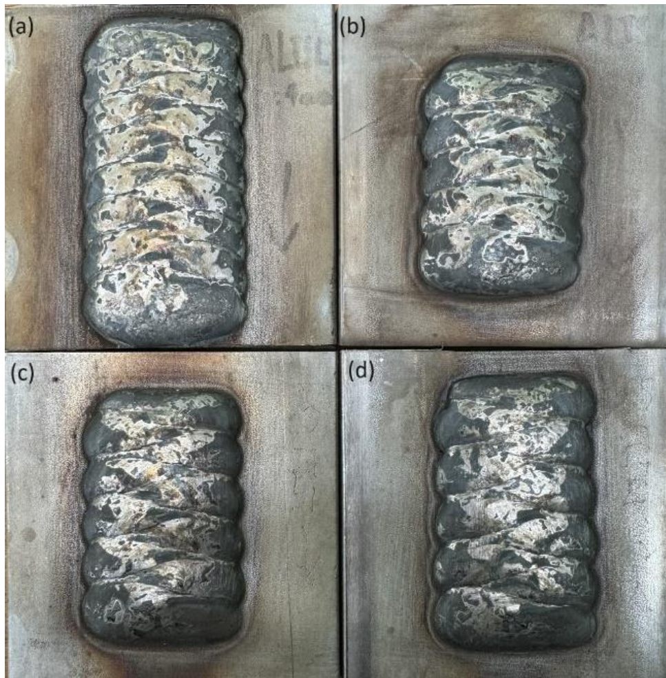
Figure 25 Rectangular weaving with different lengths of the short lines parallel to the printing direction: (a) 4 mm; (b) 4.5 mm; (c) 5 mm; (d) 5.5 mm.
