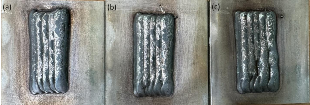
Figure 23 Unidirectional printing with different line spacing: (a) 4.4 mm; (b) 4.6 mm; (c) 4.8 mm.
