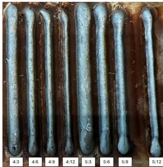
Figure 20 Lines printed with different combinations of WFR and TS. The numbers indicate WFR : TS in m/min and mm/s, respectively.
