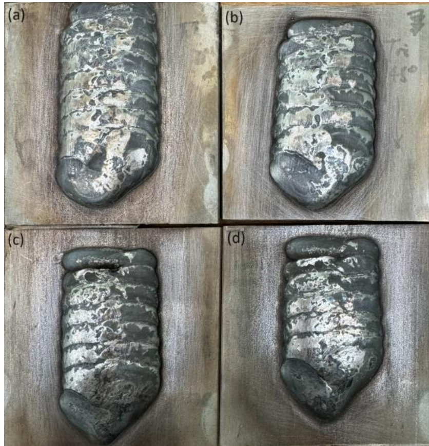
Figure 28 Triangular weaving patterns with different angle between the base and the sides of the triangles: (a) 40°; (b) 45°; (c) 50°; (d) 55°.
