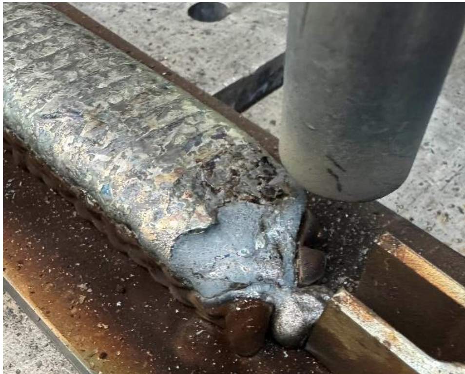
Figure 40 Collapse at the end of a layer due to the triangular shape in triangular weaving.
