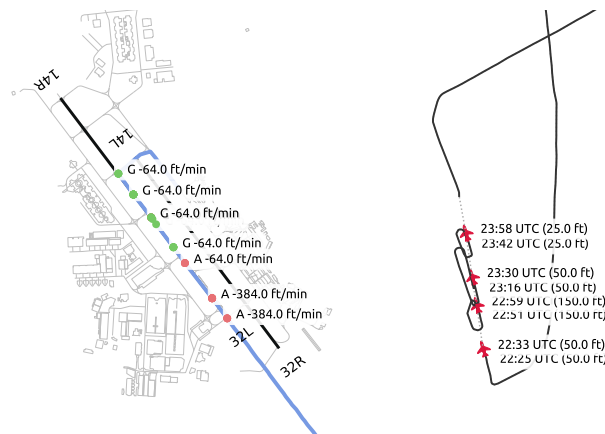
Figure 2. (Left) Flight DLH83K on 25 February 2017: it is very difficult to determine the exact landing point: the onground flag was activated after the vertical rate came close to zero. A long landing in this situation is not unreasonable, but these data cannot reasonably support this hypothesis. (Right) No onground flag is activated, but the trajectory of aircraft identifier ae0455 on 14 September 2020 suggests landing practice activity on an aircraft carrier off California.
