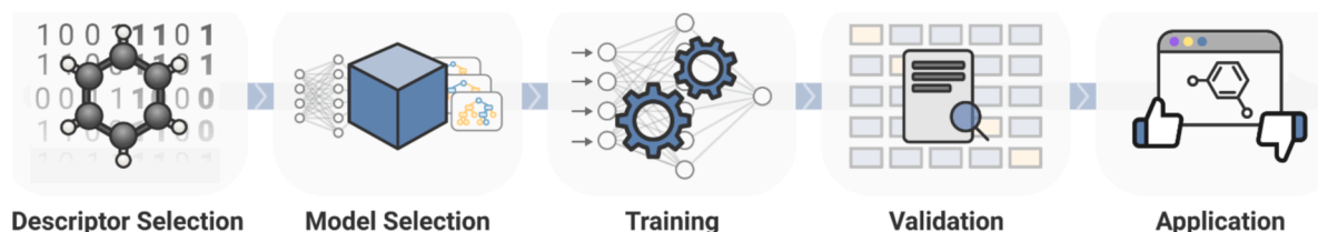
Fig. 27. Steps involved in QSPR modelling using statistical or machine learning methods.
