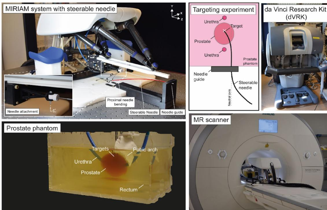
**Fig. 2** System components and schematic of the targeting experiment. The MIRIAM system holds the steerable needle and is placed in the 1.5 T MR scanner. The da Vinci Research Kit (dVRK) is placed outside the MR scanner room and the operator controls the MTM of the
