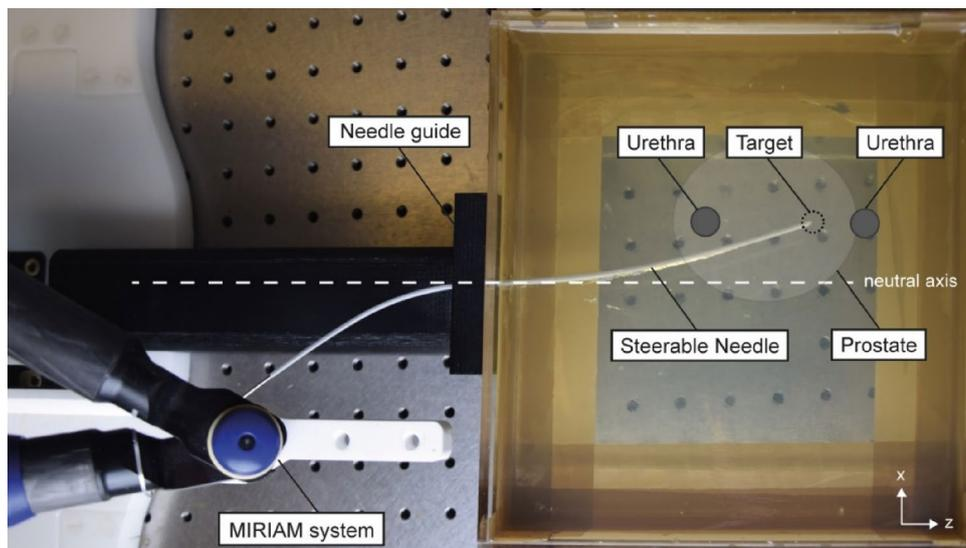
adaptations of the input position for the MIRIAM system were allowed during insertion to accurately reach the target. Figure 4 shows an example of steering with the steerable needle attached to the MIRIAM system.
