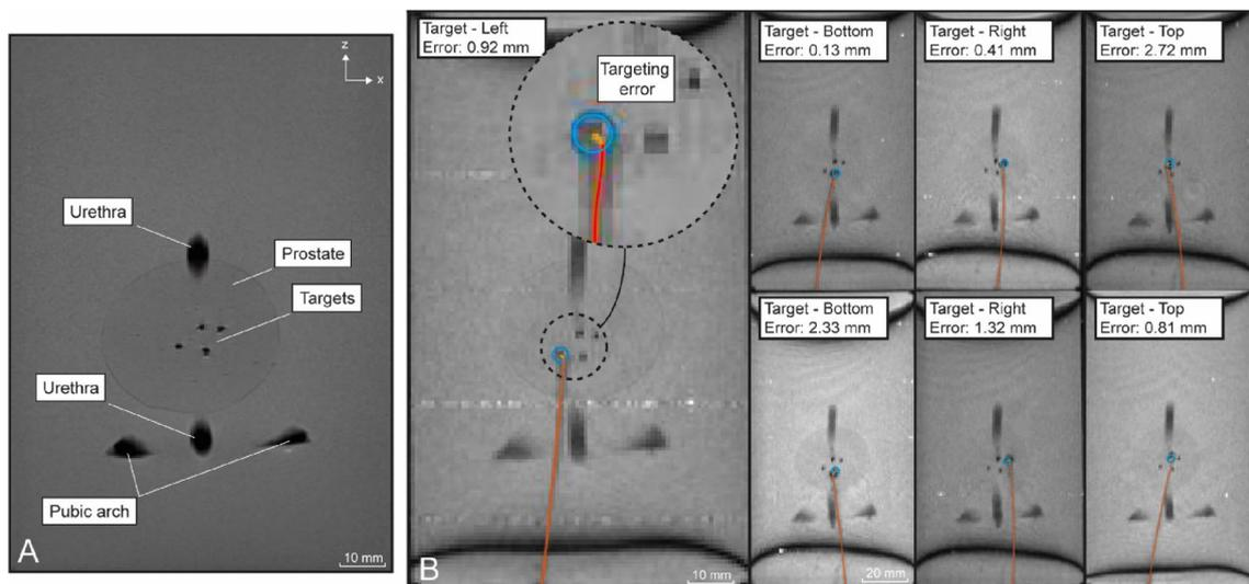
**Fig. 5** MR scans in coronal plane of the inserted steerable needle in the prostate phantom. The opacity of the prostate is changed for visualisation purposes. **A** High resolution MR scan, **B** Real-time MR
