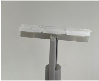
Figure 31: The suction tips placed on the suction surface. The suction tips fit exactly on the cut-outs of the suction surface.
