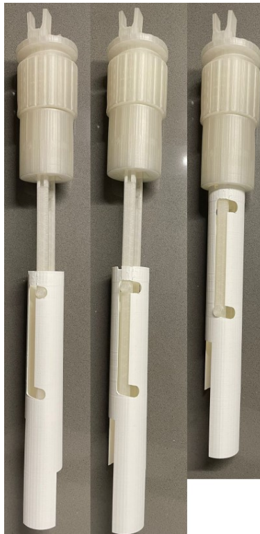
Figure 66: The 3D-printed proof of principle for the push - pull mechanism and the tensioning mechanism.
