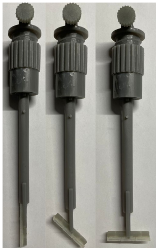
Figure 38: Prototype that is used to test the tensioning mechanism and the rotation of the suction surface. By turning the rotation knob the suction surface can be rotated.
