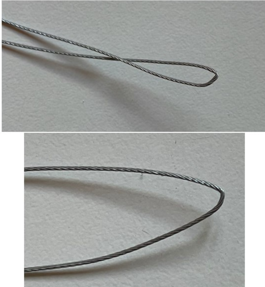
Figure 67: Cable buckling after tensioning using the prototype. The buckling prevented the cable from moving around the axis.
