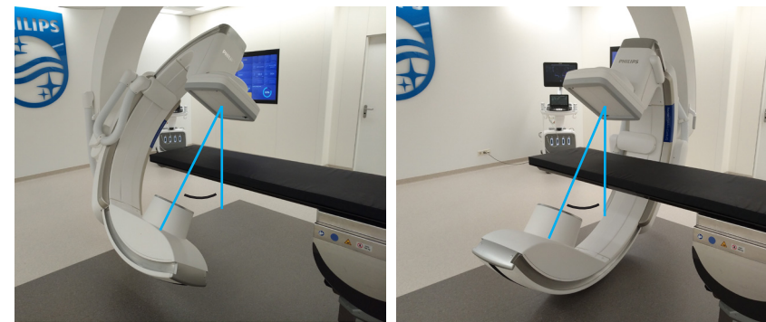
Figure 14.1.6 Difference in machine orientation for same rotation angle. Rotation around central axis on the left and Sliding in the mechanism on the right.
