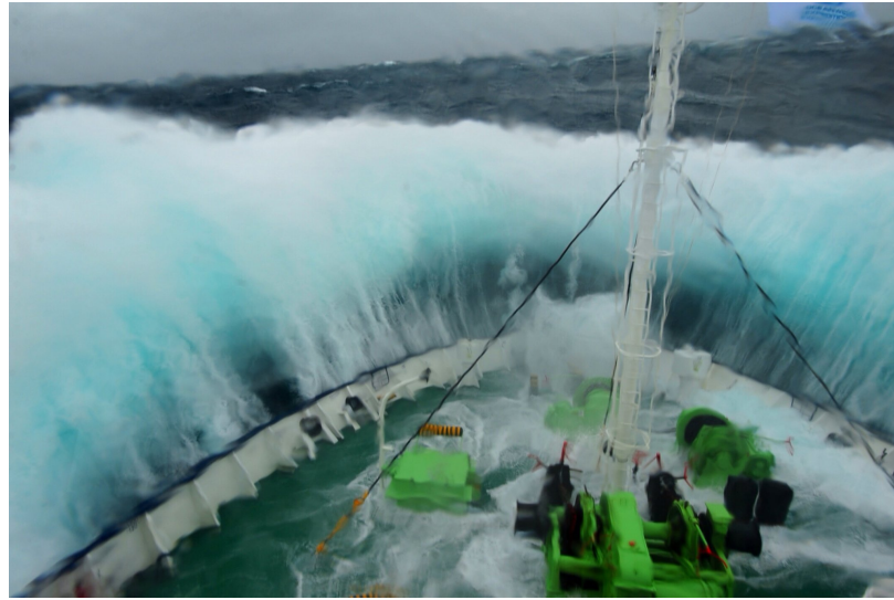
FIGURE 3.1. Green water event after slamming [250].
