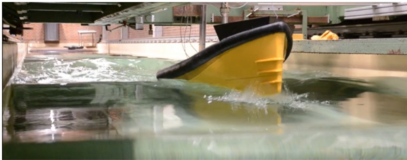
(A) Towing tank experiment of the RIB in irregular waves.
