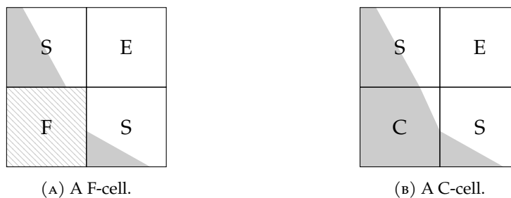
FIGURE 4.2. Difference in labeling between F-cells (left) and C-cells (right). The grey area represents the geometrical reconstruction based on the fill ratio of the cells. Fluid is indicated by ■. The F-cell is not reconstructed and therefore illustrated with a hatched pattern representing a mixture of liquid and gas. New are the C-cells in which the free surface is reconstructed for a smoother interface between fluids.
