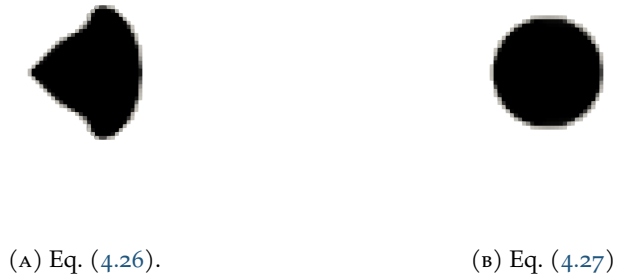
FIGURE 4.11. Comparison of the effect of using Eq. (4.26) and Eq. (4.27) on the free surface deformation. Black indicates volume fraction C_f equal to one. White indicates volume fraction C_f equal to zero.
