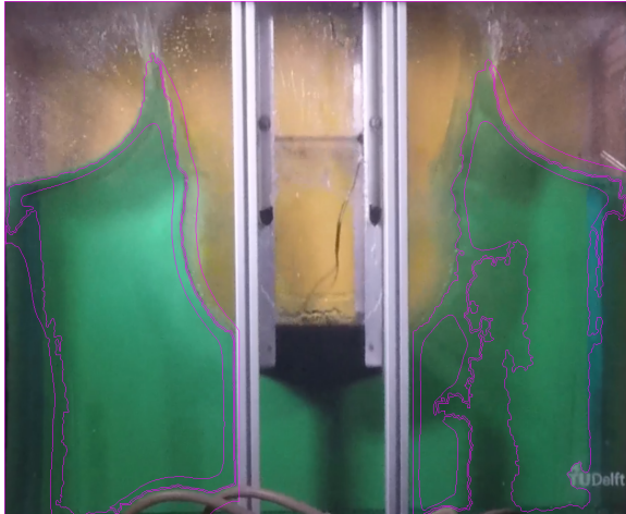
(A) Contour of the free surface in test with wedge \mu = 2.0 at 0.08[s] in closure stage.
