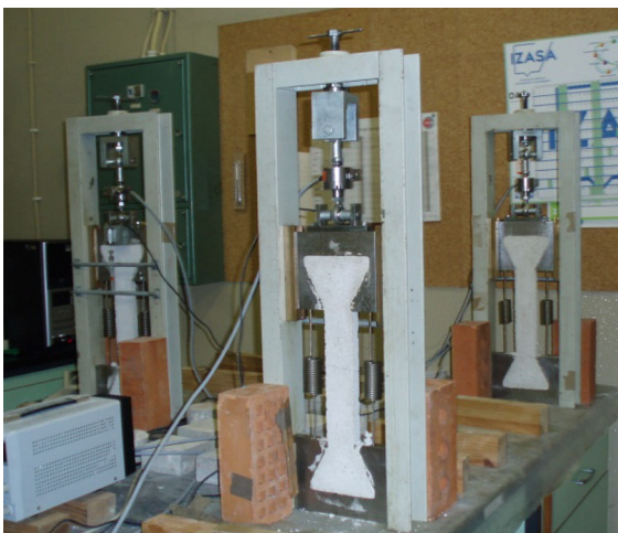
Fig. 11 Uniaxial restrained shrinkage test
