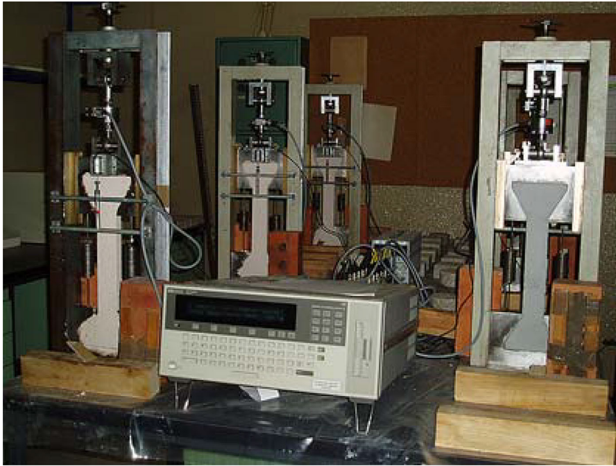
Fig. 15 Set of restrained shrinkage apparatus during a test
