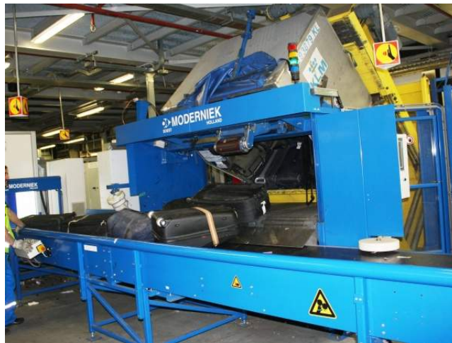
Figure 3.1: Mechanical Unloading Machine (MUM) by Moderniek D.V.
