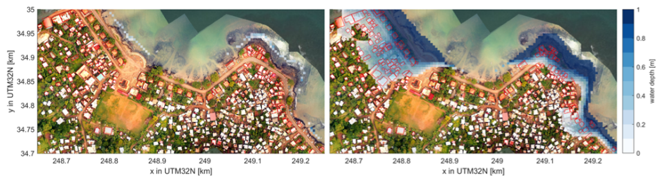
Figure B.6: Maximum computed inundation depths in Pantufo with the reference scenario (left) and for the increased water level scenario (right) with TerraSar.
