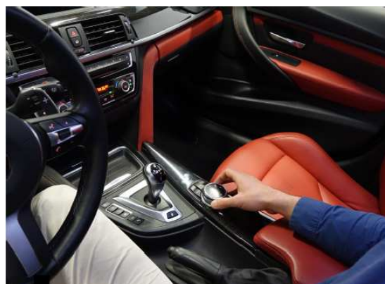
(b) A participant using the rating knob inside the simulator to rate the Perceived Motion Incongruences (PMIs), resulting in the Motion Incongruence Rating (MIR), adapted from Ellensohn, et al., 2018.
