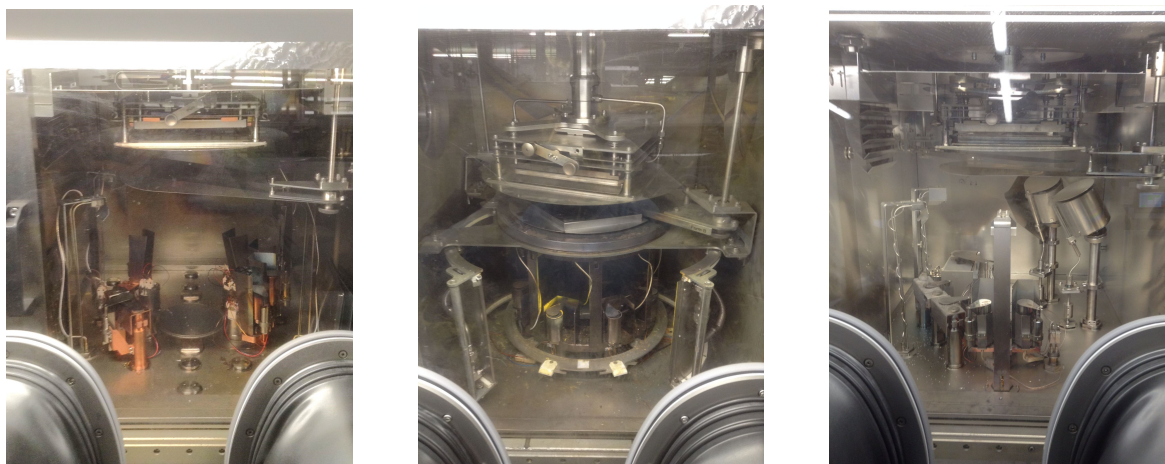
Figure 3.3: Deposition machines: OPTIvap2 (for HTL and ETL deposition), PEROVap (for PVK deposition) and OPTIvap1 (for Ag deposition).
