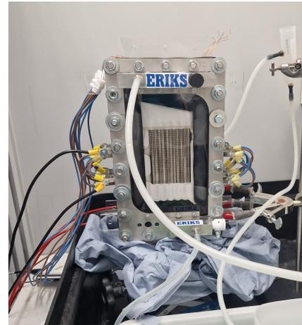
**Figure 3.7:** A frontview of the built 5-cell electrolyser stack. ERIKS, a specialized industrial service provider that offers a wide range of technical products, was the main sponsor of this project.
