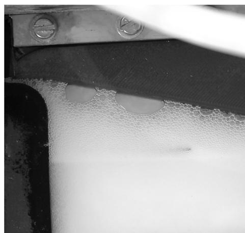
**Figure E.20:** Image of the Cathode side at liquid flow rate: 46.88 mL/min
