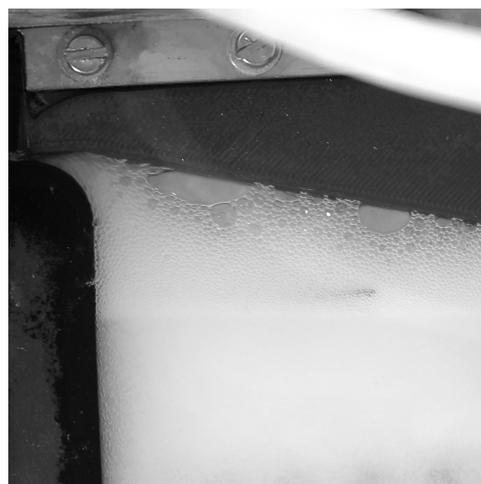
**Figure E.22:** Image of the Cathode side at liquid flow rate: 70.32 mL/min
