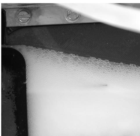
**Figure E.23:** Image of the Cathode side at liquid flow rate: 82.04 mL/min
