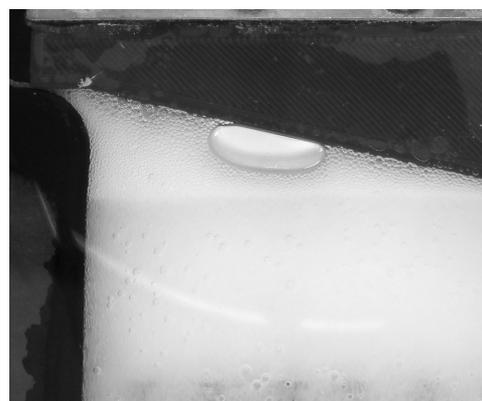
Figure E.53: Image of the Anode side at gas flow rate: 88 mL/min
