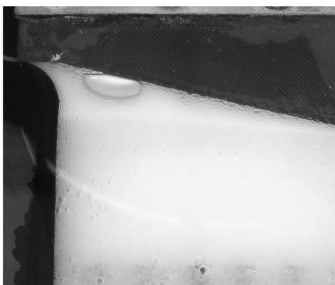
Figure E.52: Image of the Anode side at gas flow rate: 78 mL/min
