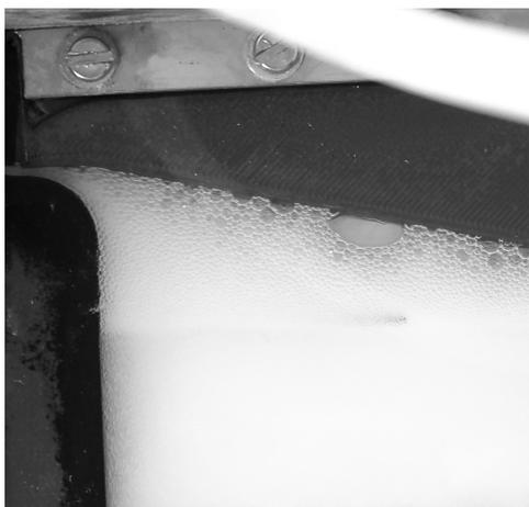
**Figure E.21:** Image of the Cathode side at liquid flow rate: 58.60 mL/min
