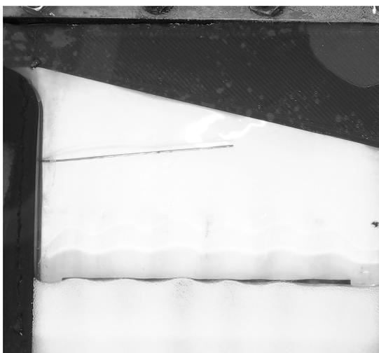
**Figure 4.8:** An in situ image of the anode compartment at an electrolyte flow rate of 0.596 mL/min and a  $O_2$  gas flow rate of 78 mL/min per cell. This  $O_2$  gas flow rate is achieved at a current density of 278 mA/cm<sup>2</sup>.
