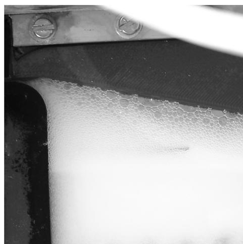
**Figure E.24:** Image of the Cathode side at liquid flow rate: 93.76 mL/min
