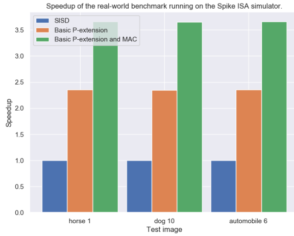
Figure 5.7: Speedup when using the SIMD instructions of the P-extension for the different images in the Cifar-10 benchmark running on Spike.
