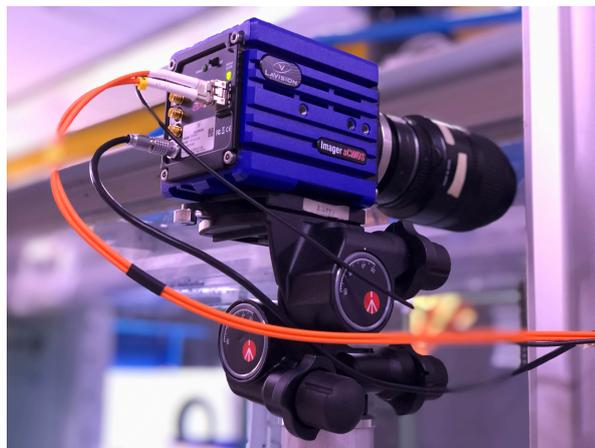
Figure 3.6: sCMOS camera by LaVision with  $105 \text{ mm}$  focal length Nikon objective.
