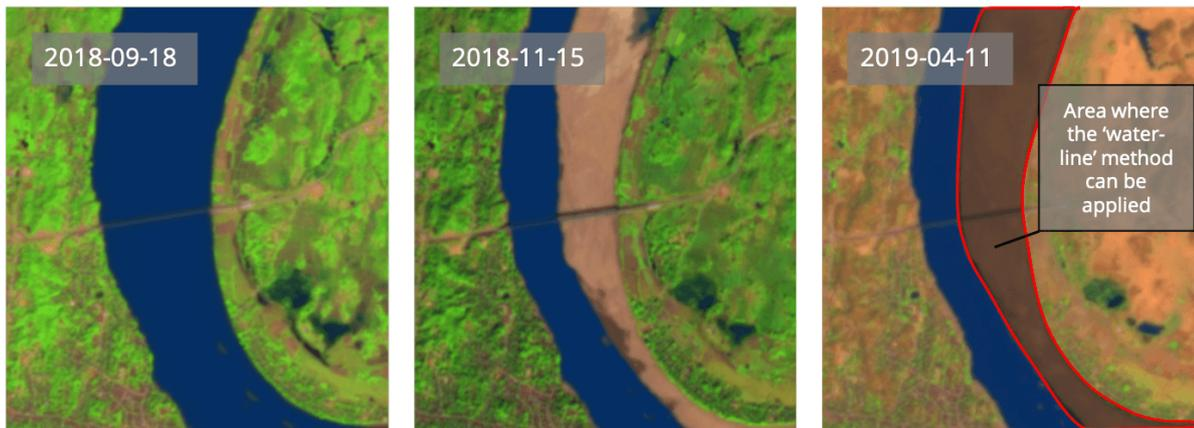
Figure 2.10: False colour images near Kalewa Bridge. The left image is taken during the monsoon period, the middle shortly after and the right image is taken approaching the end of the dry period. The red line displays the area of the river where the 'water-line' method can provide information about the bathymetry
