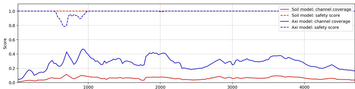
Figure 3.22: Performance indicators for a stretch of the river near Kalewa. Calibration factor  $a = 5$ , bank full water level = +8.0 m.
