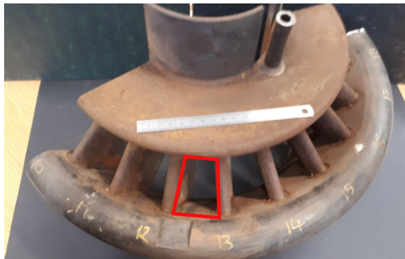
Figure 6.7: Top view of the HR3 burner. The picture is taken by Uniper.
