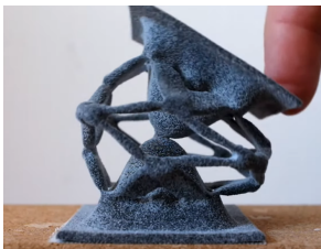
(a) Example of a prototyped flexure of which the stiffness of the degree of freedom remains relatively constant over a larger range of motion.
