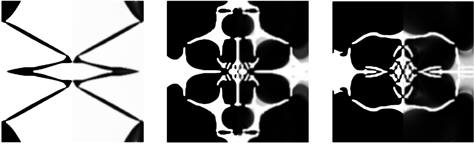
Figure 7.1: Various solutions to the problem formulation as proposed by Koppen et al. (2021b) (maximization of shear stiffness ( \tau_y ), subjected to maximum axial stiffness ( \tau_x )) without volume constraint for various ratios of solid to void stiffness. From left to right these ratio is 1 \times 10^3 , 1 \times 10^6 and 1 \times 10^9 , respectively. For each of those solutions the filtered design variable field is displayed on the right side; a post-processed design interpretation is displayed on the left.
