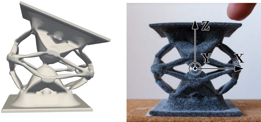
Figure 2.1: Computational design of a multi-axis flexure and its prototyped counterpart. The flexure is compliant in the rotations about the x and y -axis while stiff in the x , y and z translations as well as rotation about the z -axis.
