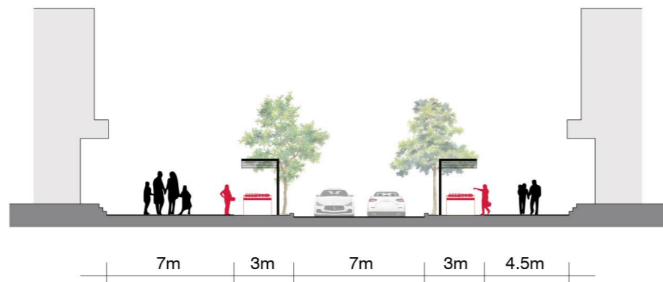
Fenghua road section
