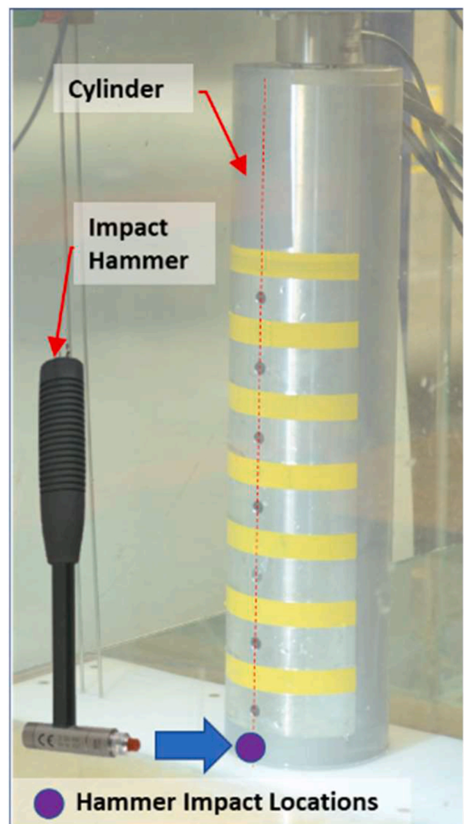
Fig. 14. Impact hammer tests and impact location.
