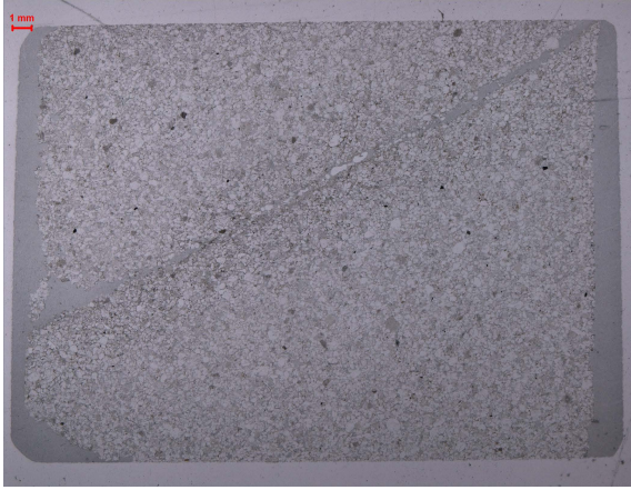
Figure 28: Thin section image of BS-09 under polarized light
