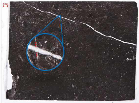
Figure 32: Modified thin section image of TM2-2 under polarized light with enhanced contrast and brightness. The magnification marks the very limited fracture offset.
