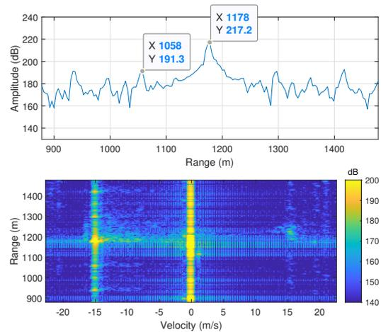
Fig. 10. Matched filter response for moving target; range and range-Doppler map
