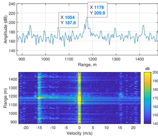
Fig. 9. Decirping and decoding with reference delay  $R = 50$  m for moving target; range and range-Doppler map
