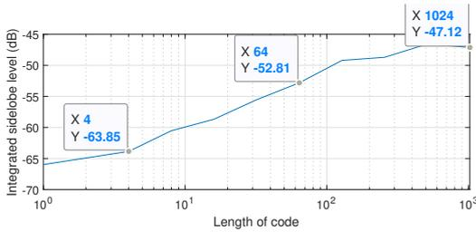
Fig. 3. Integrated sidelobe level vs the code lengths
