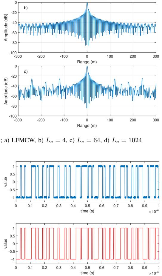
Fig. 5. Received communication signal; after band-pass filter (blue), after threshold (red)
