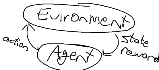
Figure 3.1: The interaction between an agent with its environment in a Markov Decision Process
