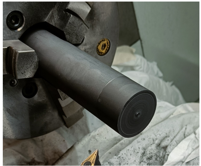
(b) Graphite nozzle in the process of being machined.
