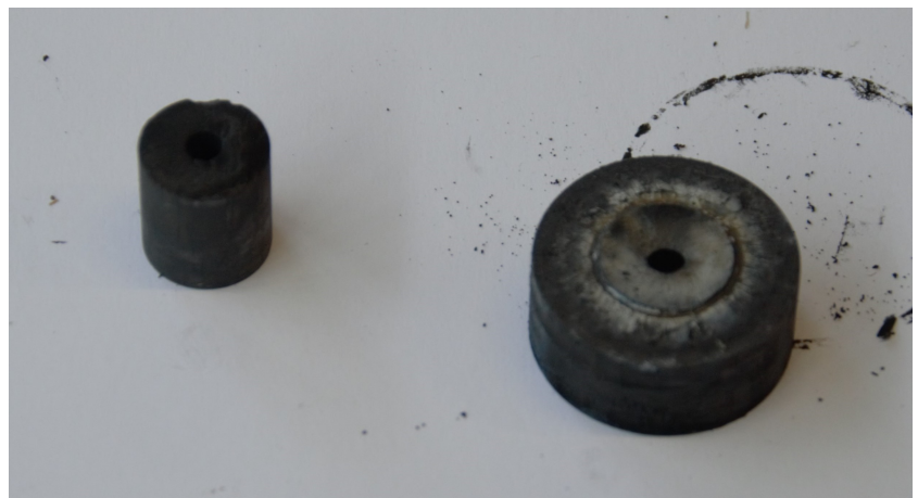
(b) Forensics image of a graphite nozzle with the divergent section broken off during a motor test during the first test.
