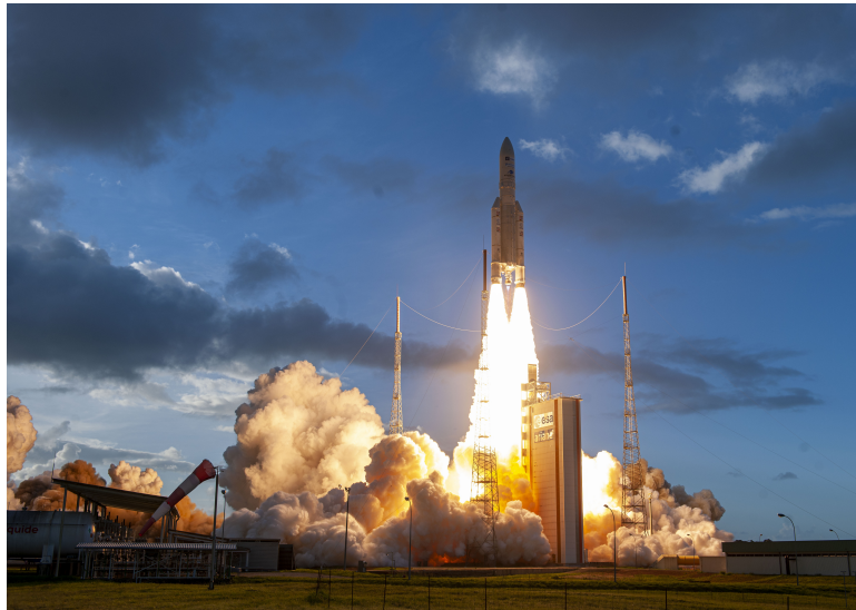
Figure 1.1: Image of ESA's Ariane 5 rocket taking off with two SRMs as side-boosters. Image credit: ESA/CNES/Arianespace.
