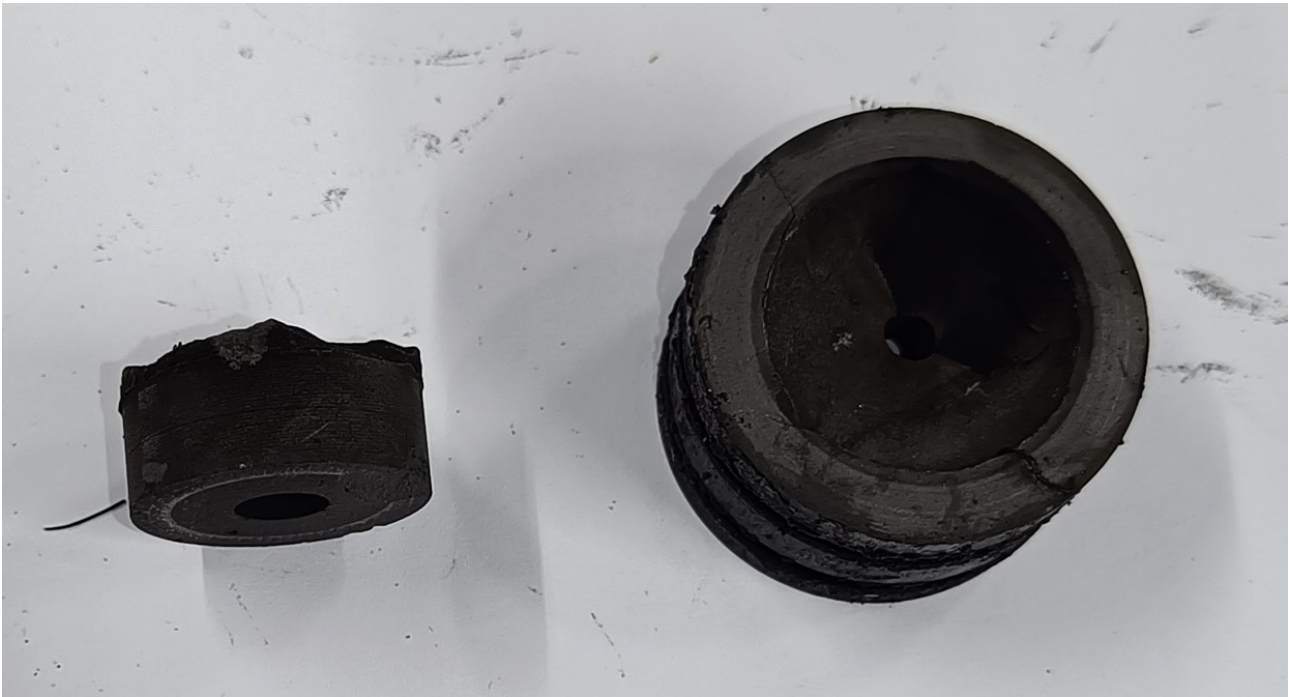
Figure 3.14: Broken graphite nozzle from double hole test 2.
