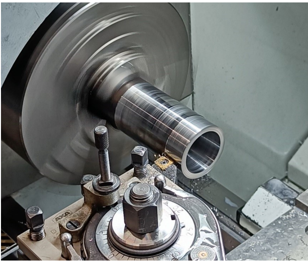
(a) One of the motor casings in the lathe.
