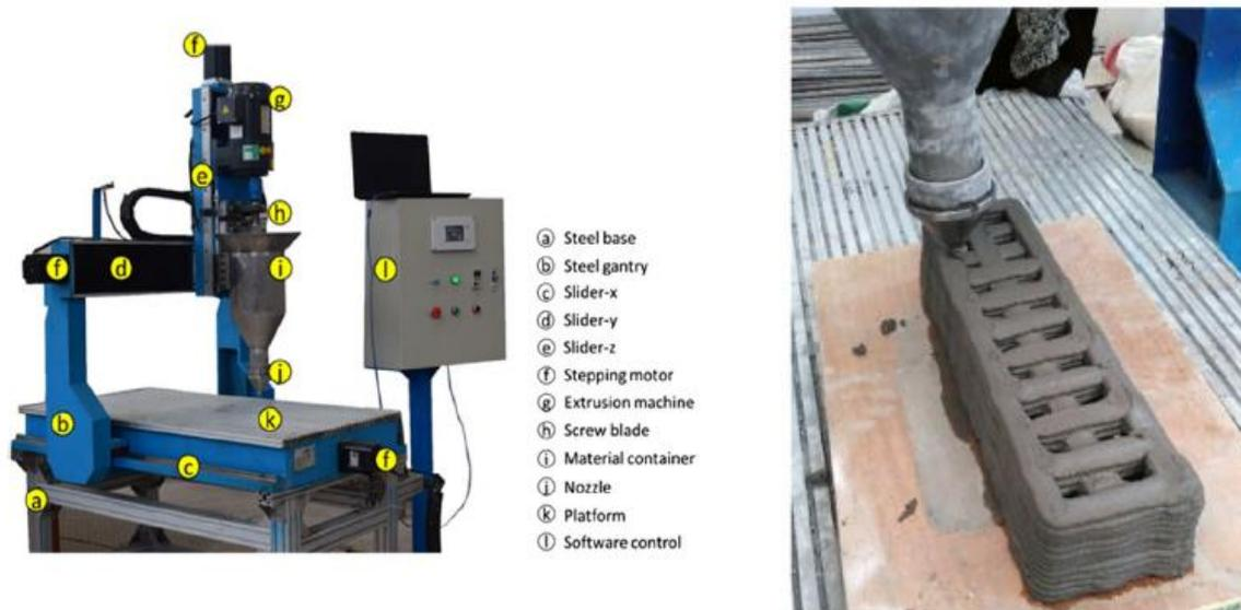
Figure 2-5 The demonstration of extrusion-based printer for cementitious material (left) and the example of lattice-shaped hollow section specimen under the printing process(right) [54]
