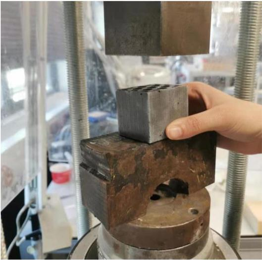
Figure 4-3 Left: The operation of manual hydraulic press. Right the detailed demonstration of specimen
