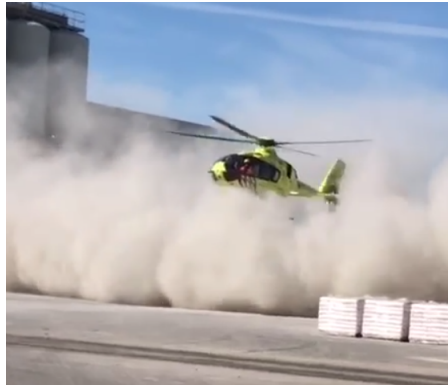
Figure 9.1: Dust 'brown out' of a helicopter. Footage Courtesy of HEMS Pilot G. Ruitenber
